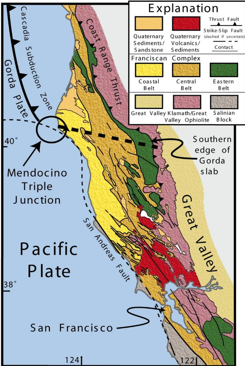
**Figure 3** Simplified geologic map of northern coastal California. Young volcanic rocks north of San Francisco Bay locally overlie the three belts of the Franciscan Complex. Primary crustal thickening occurs within the Central belt of the Franciscan Complex between 40°N and 41°N.
